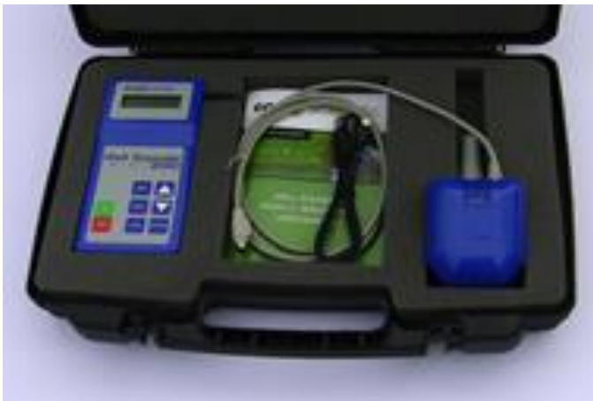
Figure 2: Portable well sounder probe (Eno-Scientific 2010) [16]
